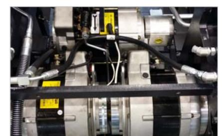
**IP43 dust and water protection Drive and Pump**
